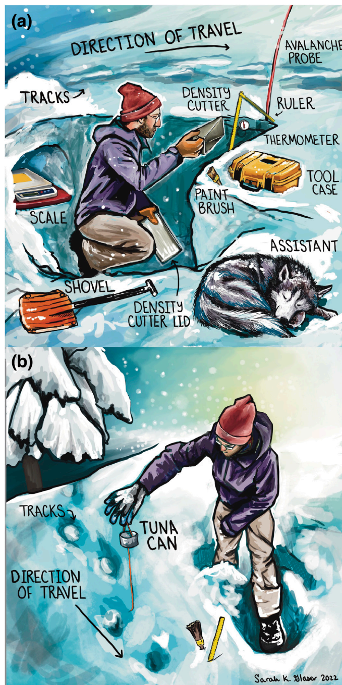
Figure 2. Illustration of field sampling protocol. We excavated a snow pit parallel to the animal's direction of travel and conducted observations, including measuring density of the top 30 cm (a; AvgDens ), determining hand-hardness across the full pit's depth ( AvgHH ), quantifying thickness and depth of ice layers ( IceTop and TotalIce ), and measuring surface penetrability via tuna can drops (b; AvgTuna ). The string under the tuna can measured 50 cm, the height at which the can was dropped from. Illustration by Sarah K. Glaser.
